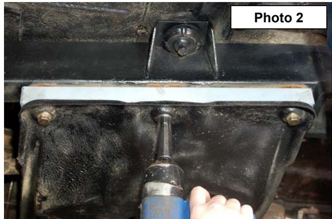
6. Using the conical bolts supplied slightly tighten the bolts. **Do not fully tighten** to allow for some movement for the opposite side.
