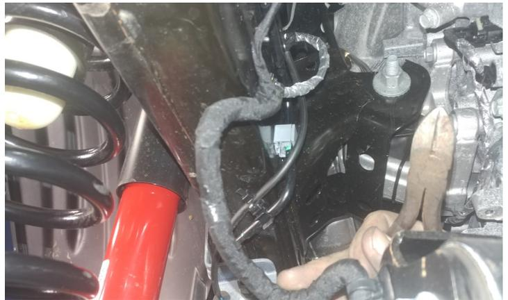
Locate the wire harness on the driver side frame rail and pull all clips out of the frame. Allow the harness to hang out of the way.
