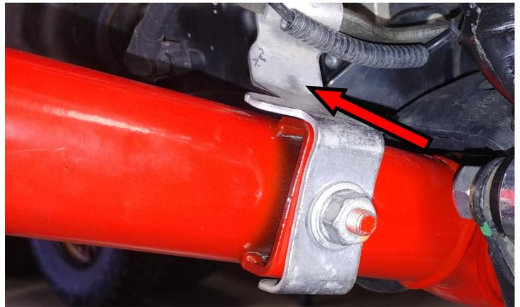
Install the electrical connector that was previously cut to the lower hole in the frame rail. The rest of the harness will hang.
