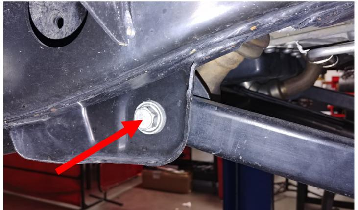
Loosen the **front lower control arm hardware at the axle**. Do not remove at this time.
