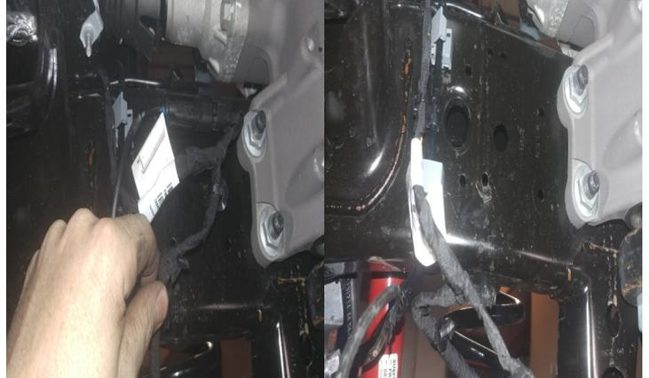
Using a suitable cutting device, clip the outside "Christmas tree" nipple off the electrical connector.
