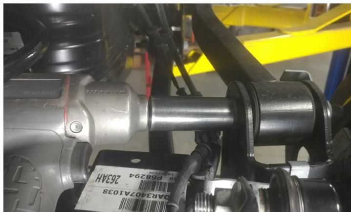
Loosen but do not remove the rear lower control arms at the axle and frame.
