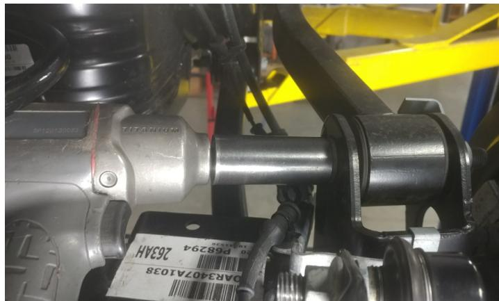
Loosen the rear track bar at the axle and frame.
