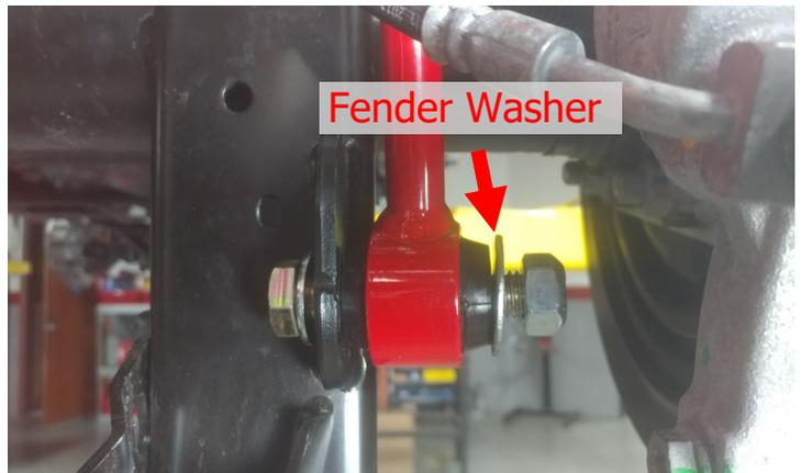
Attach the ReadyLIFT brake line bracket to OE bracket using the provided 1/4" x .75" bolt, washers and nut. Gently rotate/bend the metal brake line. Install using the factory hardware. Torque all to 5 ft-lbs.
