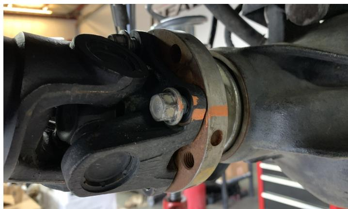
Remove the front drive shaft from differential. **Caution** do not let the drive shaft hang this may result in damage to the rear seal. Place the drive shaft on top of the differential or use a hanger.
