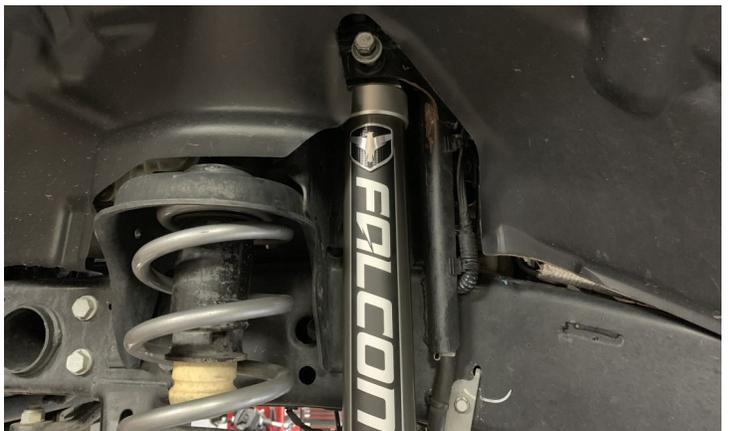
Install the **11" replacement end links** to the sway bar using supplied **1/2" bolt, fender washer, flat washer and nut** on the sway bar. Be sure to install the fender washer to the outside of the end link. Install the axle side of end link using **factory hardware**. Torque to **45 ft-lbs**.
