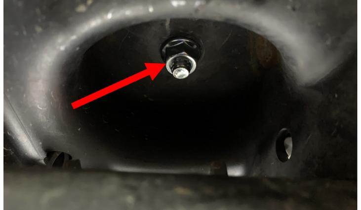
With bump stop hardware torqued install the brake line bracket on the axle.
