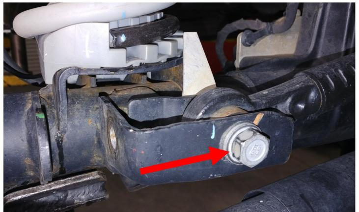
Remove the **front track bar bolt at the frame**. Retain factory hardware. Remove complete track bar assembly from vehicle and discard.
