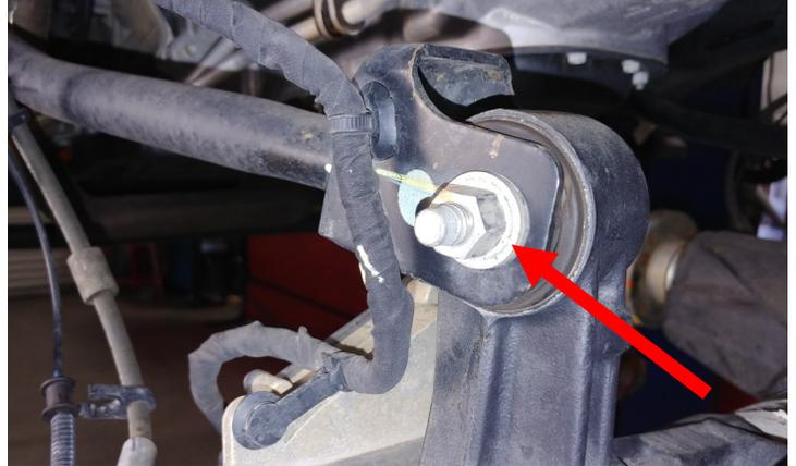
Loosen the **front lower control arm hardware** at the frame. Do not remove at this time.
