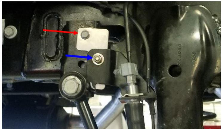
Install the wheels and lower the vehicle to the ground. Torque the lug nuts to the wheel manufacturer specs. Jounce the vehicle a few times to settle the suspension to the new ride height. Torque the upper control arms to **135 ft-lbs**, lower control arms and track bar hardware to **135 ft-lbs**, and shock and sway bar end link hardware to **50 ft-lbs**.
