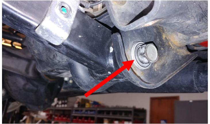
Remove the front shock from vehicle at this point and discard. Retain upper mount factory hardware.
