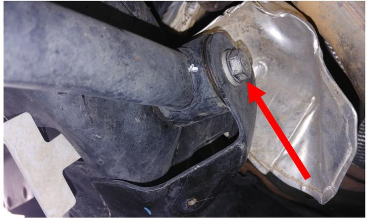
Loosen but do not remove the **front upper control arm bolts** at the axle.
