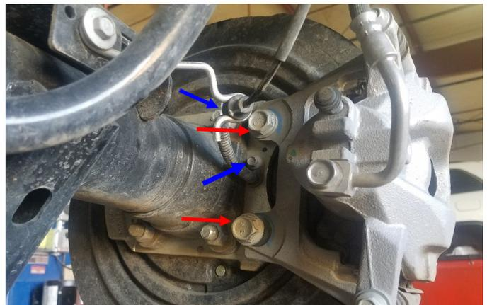
Remove the rear upper and lower shock bolts. Remove factory shock from vehicle and discard. Retain factory hardware.
