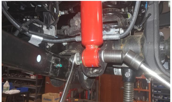
Remove the **front track bar hardware at the axle**. Be sure to retain factory hardware.
