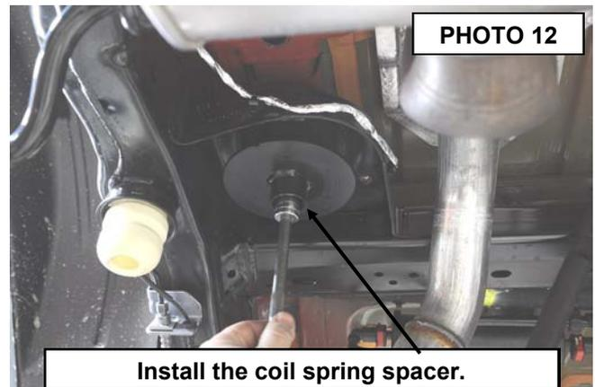
**Install the coil spring spacer.**
