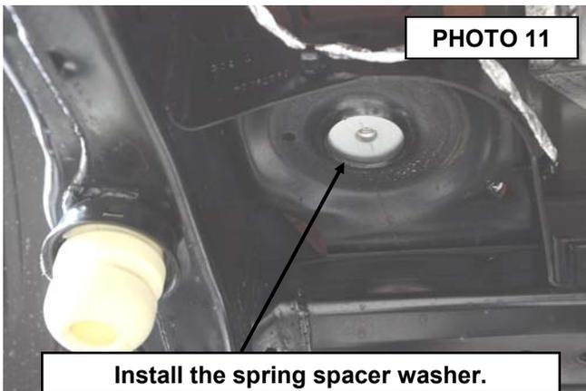
**Install the spring spacer washer.**
