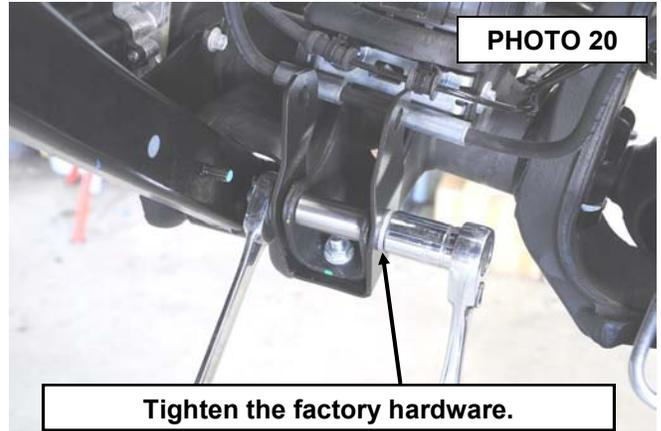
24. Tighten the lower shock bolt using an 18mm socket and wrench. Torque to 55ft/lbs. **See Photo 21.**
