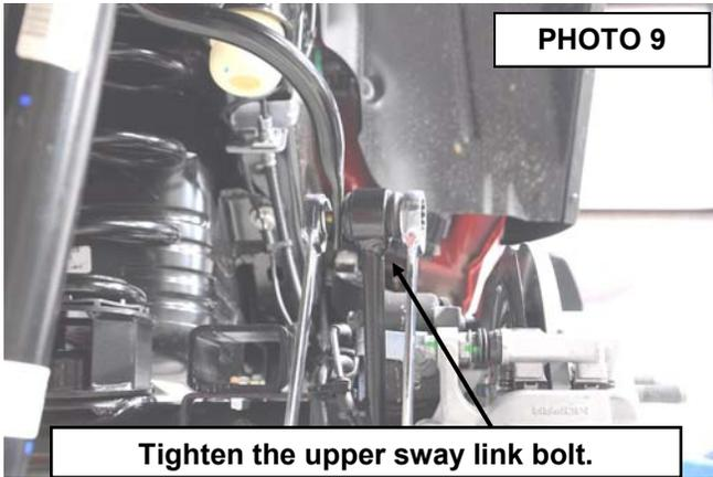
**Tighten the upper sway link bolt.**
