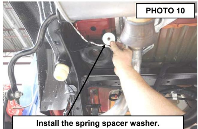
**Install the spring spacer washer.**
