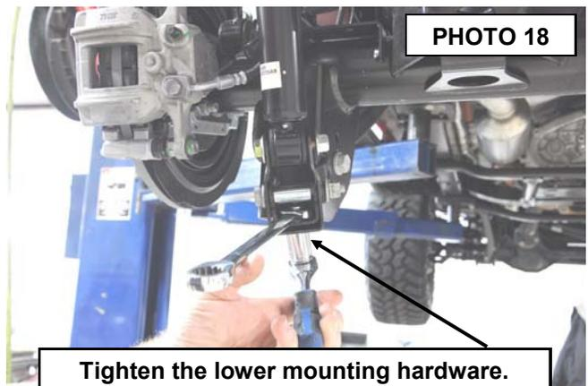
21. Install the sway bar links, in the lower mount using the factory bolts and an 18mm socket and wrench. Torque to 55ft/lbs.
